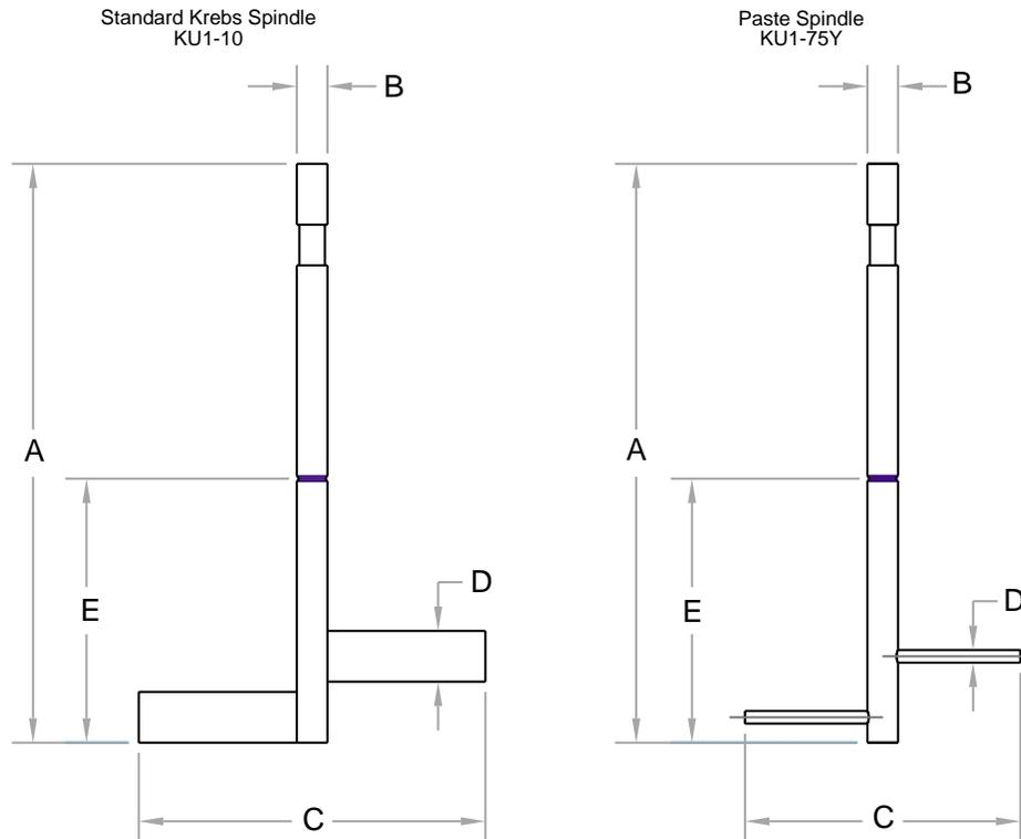
The KU-2 (KU-1+, KU-1) Viscometer measures viscosity in Krebs units and grams. The KU-2 Viscometer also reports the viscosity reading in centipoise. The measurement is made by rotating the spindle at 200 rpm.
