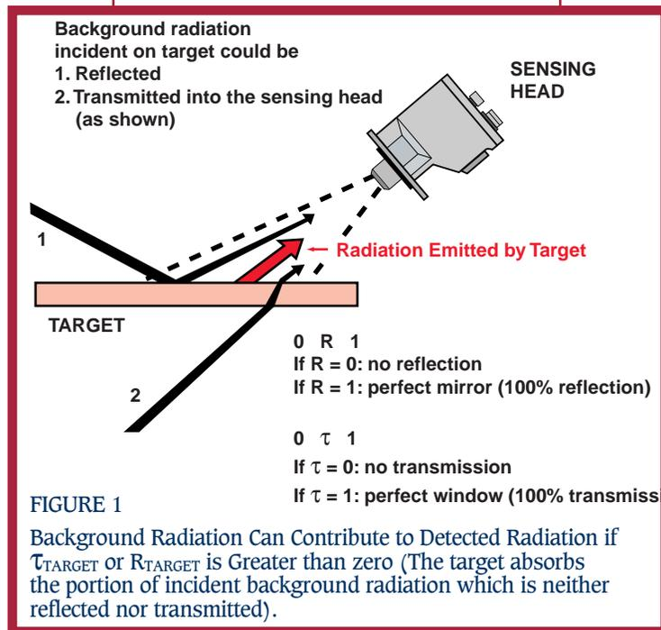
infrared radiation, it is impossible to know if background radiation is significant enough to produce an effect. We can estimate the significance of the background's radiance, relative to the target's, simply by comparing the approximate temperatures of the target and background sources.
