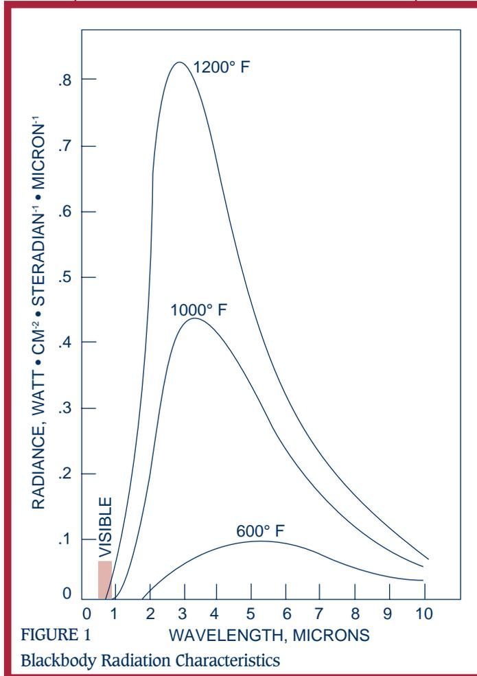
cannot see it. However, there is still copious emission of infrared radiation. Note that the radiance at every wavelength increases as temperature increases, and that the determination of the radiance at any wavelength can serve to establish the emitter's temperature.
